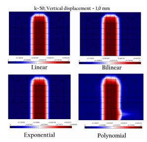
Figure 7. Evolution of damage to the four damage functions: vertical displacement of 1,0 mm.
